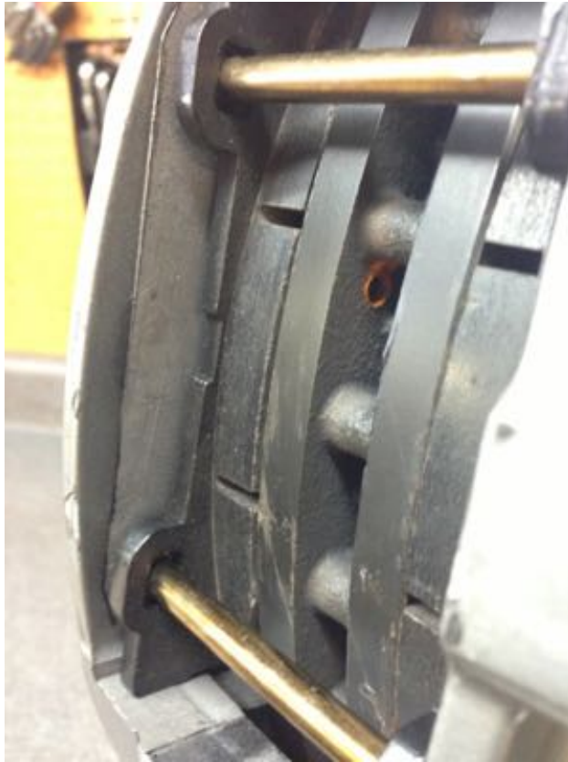
Figure 6: Proper Pad Contact
