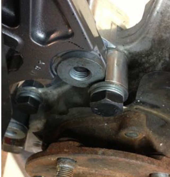
Figure 3: Slotted Washer in Position with Caliper Installed
