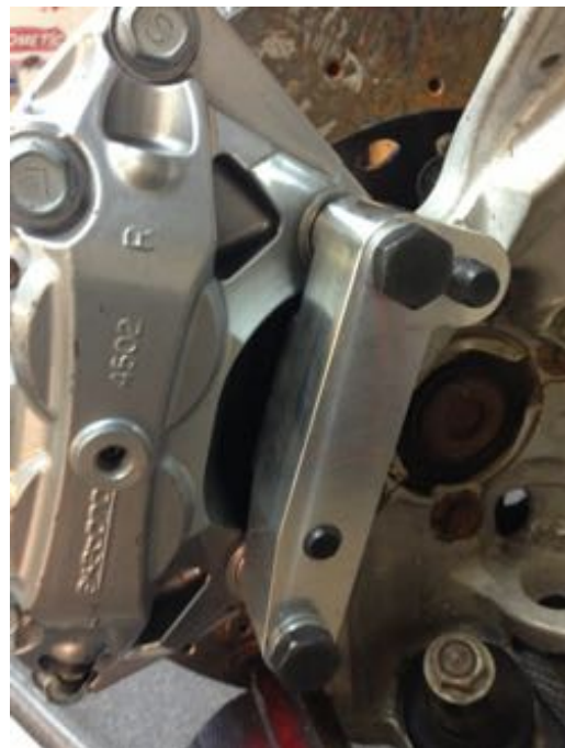
Figure 5: Caliper bolted to Adapter Bracket – Rear View
