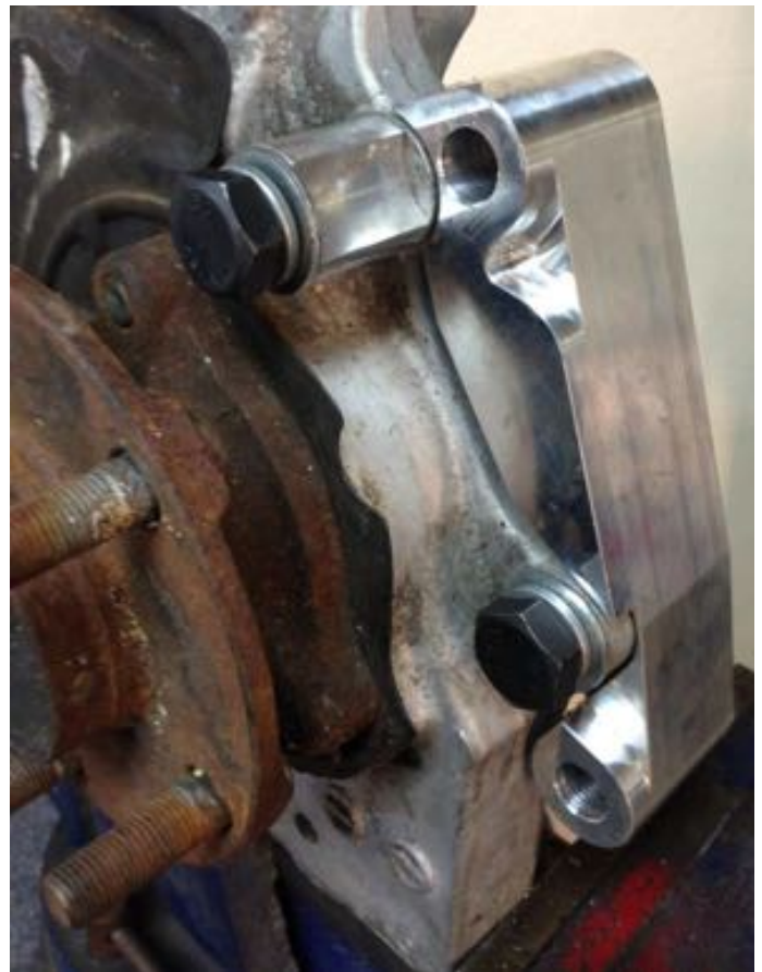
Figure 2: Bolts and Washer Holding Adapter
