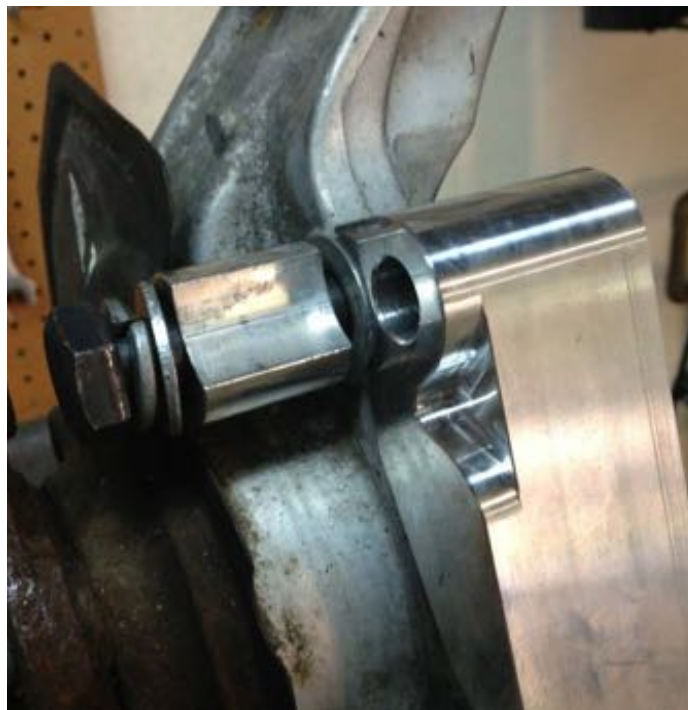
Figure 7: Slotted Spacer Assembly Order: 90mm bolt, lock washer, flat washer, slotted washer to spindle
