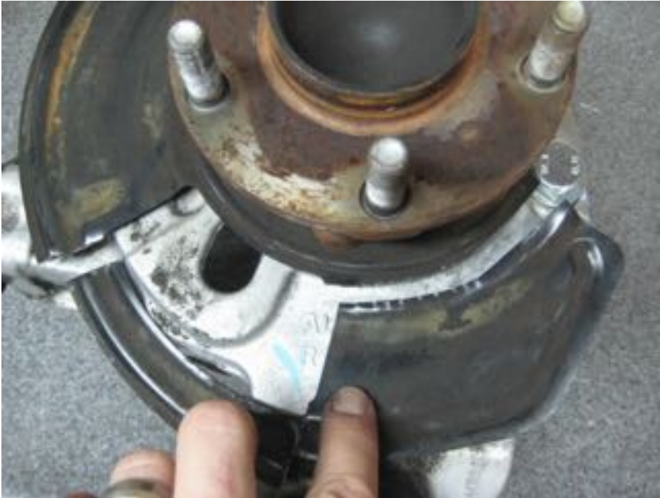
Figure 9: Heat Shield Section to Remove
